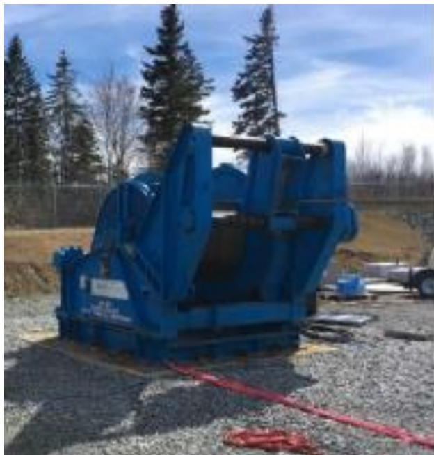
Image 9.2 Typical onshore cable pull-in winch
